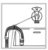
If it is placed over the edge of a basin or sink be sure the free end of the hose should not be underwater.
