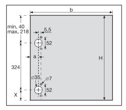
if width **(b)** increases, measurement **a** must also be increased
