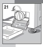
ATTENTION!! Before starting the operations described below, make sure that the washing machine is empty. Do not remove the filter while the machine is running, or when full of water.
