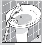
If the waste water is to be discharged into a sink or washbasin, insert the hose in the special bracket supplied and hook it over the edge of the sink or washbasin. Then tie the hose and bracket to a tap or similar (fig. 8). To avoid overflowing, the sink drain must be clear of obstructions and must be able to empty quickly.
