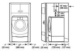
Recommended installation spacing for recessed or closet installation, with stacked washer and dryer
