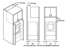
Required spacing \*\*For side or bottom venting, 0" (0 mm) spacing is allowed.
